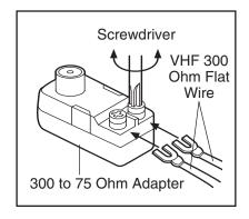
Push the 300 ohm to 75 ohm adapter onto the 75 ohm antenna terminal on the treadmill frame near the power cord.
